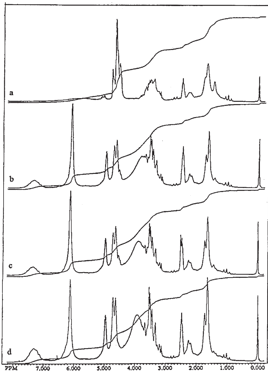
Figure 2 ^1\text{H-NMR} spectrum of 5-HMCH (prepared from 1 mol of cyclohexanone and 5 mol of formaldehyde) (a) and those of melamine solutions in the reactive solvent recorded after 3 min (b), 5 min (c), and 7 min (d) from the beginning of dissolution.
